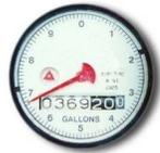
The long hand measures water and shows larger water flows. The triangular hand shows smaller water flows. Most meters have a 7 digit number on the face which look like a car odometer.
